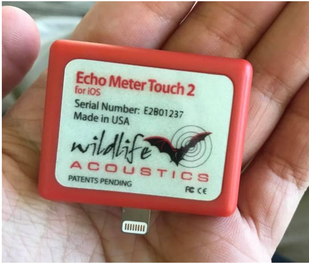
Fig. B. The Echo Meter Touch 2 bat detector, which plugs into an iPhone or iPad
